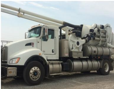
*A: This is the Town Vactor Truck, essentially a very powerful vacuum unit that sucks up debris from catch basins, storm drain lines, and sumps. The vacuum compressor produced 8,000 cfm (cubic feet per minute); a standard vacuum cleaner produces about 85 cfm. The truck also has 600 feet of 1 inch hose, to which various nozzles are attached to propel the hose up lines and bring any debris back to the manhole or catch basin for suction and removal.*
